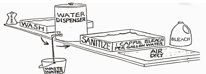
An approved method of washing preparation utensils in a booth if plumbing is unavailable.
